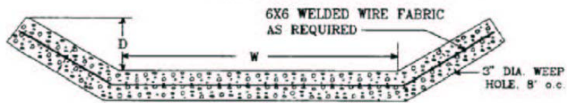
TRAPEZOIDAL WATERWAY CROSS-SECTIONS
